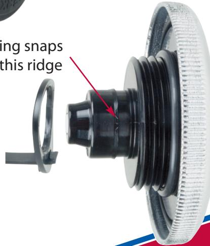
Once attached the ring allows the cap to turn freely without binding or twisting the tether.
